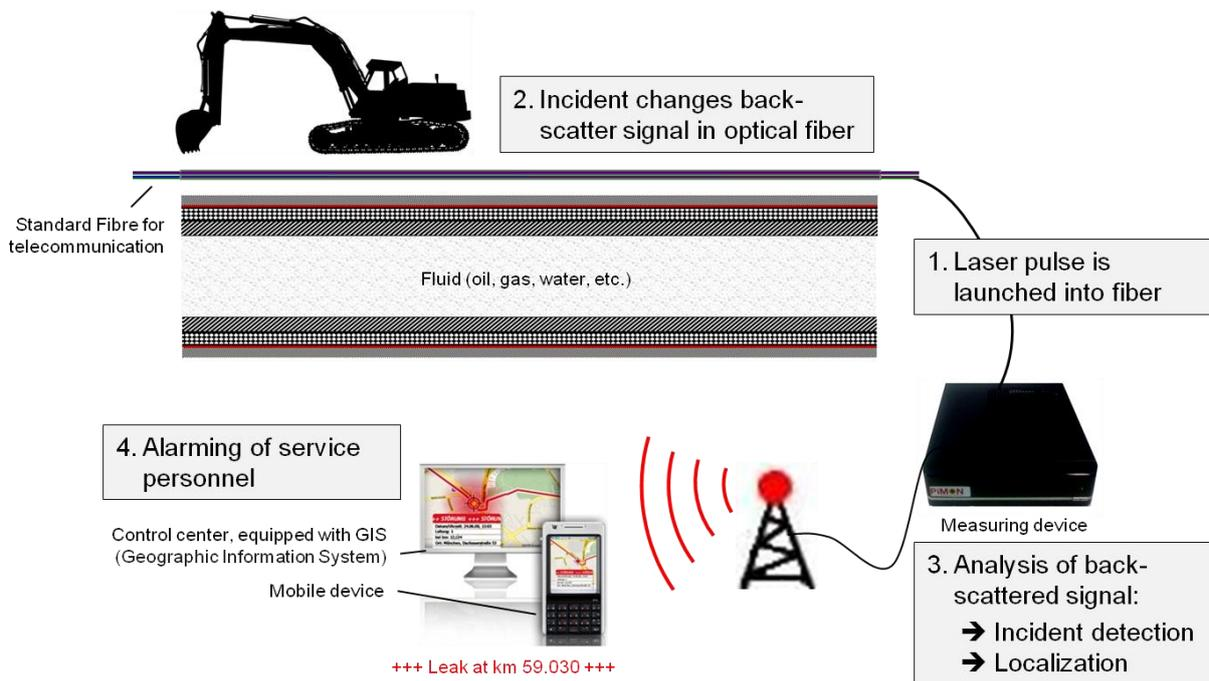
Figure 2: PiMON's Working Principle
